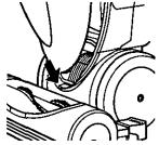
4) Replace the dust cover by inserting the protruding tab into the body slot then push the top of the cover into place
